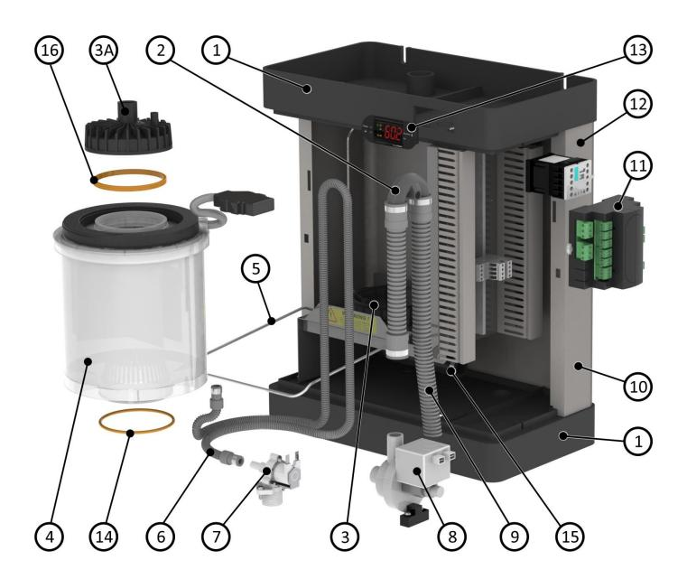
ES SERIES SPARE PARTS AND EXPLODED DIAGRAM
