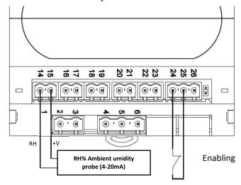
The Bp proportional band is the percentage value of the humidity around the set point; within this value the humidifier works proportionally. Example: if the proportional band is set on default value 10% (-5% / +5% set point value) and humidity is set at 50%, below 45% the humidifier will work at 100% of steam output; above 55%, the humidifier will not produce steam. Between 45% and 55%, the humidifier will optimally regulate steam output.
