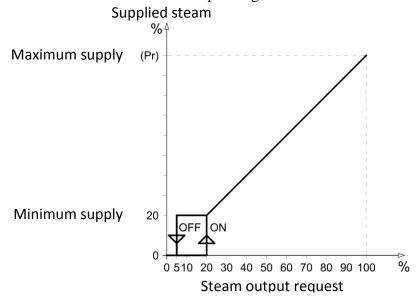
described in chap. 2.4. The minimum steam supply is fixed at 20% and is managed with an activation hysteresis; maximum supply had in correspondence with a maximum requested corresponds to the percentage set in the first level variable If, for example, on an ES6 producing 6Kg/h of Pr steam 100% is set, maximum supply will be 6Kg/h; but if Pr is reduced to 50%, maximum supply will be 3Kg/h.
